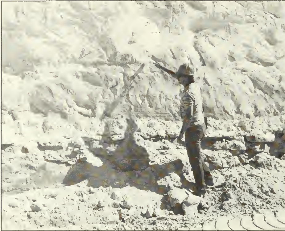
Photo 7. The working face of the Dicalite quarry (Grefco) near Lake Britton, Shasta County. The man is pointing to a 2-inch layer of sandy detritus which will be selectively removed during mining. (Photo by John L. Burnett.)
